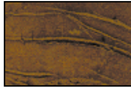
THORN SCRATCHES of that magnitude, with open hide tissue will not be used on furniture. A major quality flaw.
